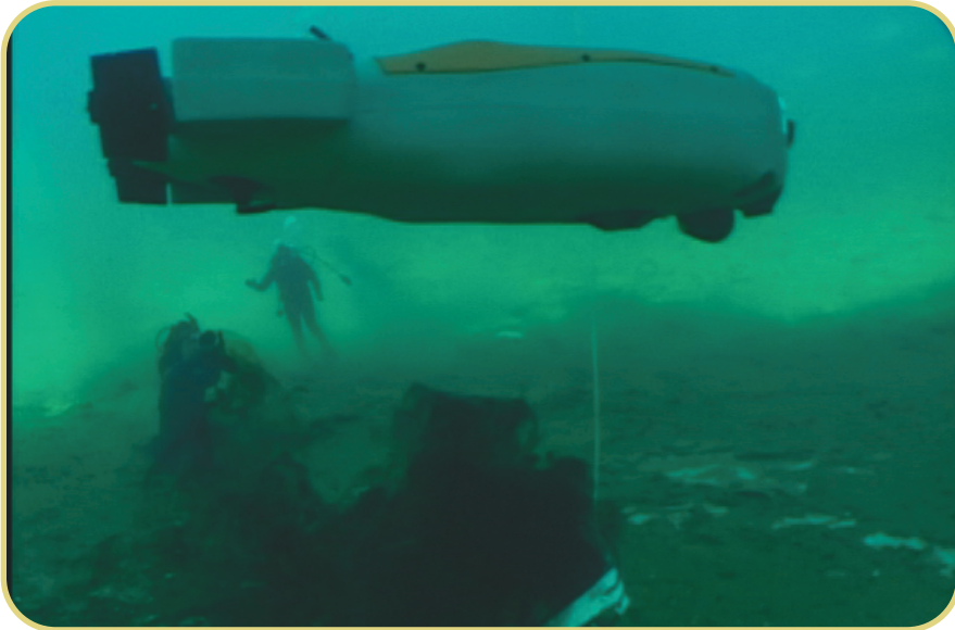
Autonomous robots such as the Cetus II are used in exploration, air crash recovery, and other hazardous underwater missions.
